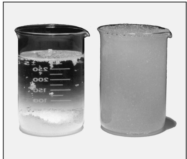
The H-400 and H-500 series polymer is slower in absorption time, but easy to apply and dispose of in its granular form.
